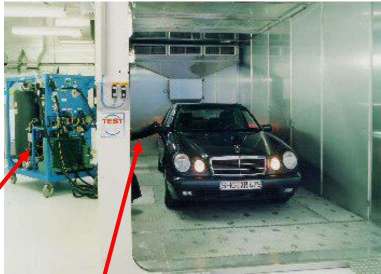
Refueling nozzle through the SHED wall—booted for operator arm (not vapor recovery)
